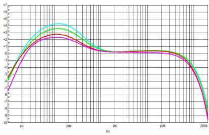
Magenta: Satuation Max Red: Saturation @ 2 o'clock Green: Saturation @ 10 o'clock Cyan: Saturation @ Min
