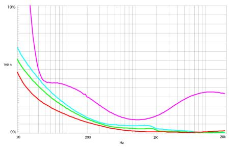
Red: Input 0dBU Saturation at Min (Drive = 2) Green: Input 0dBU Saturation @ 10 o'clock (Drive = 2) Cyan: Input 0dBU Saturation @ 2 o'clock (Drive = 3) Magenta: Input 0dBU Saturation @ Max (Soft Clipping (Drive = 6)
