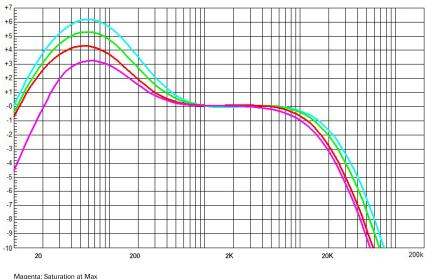
Magenta: Saturation at Max Red: Saturation at 2 o'clock Green: Saturation at 10 o'clock Cyan: Saturation at Min
