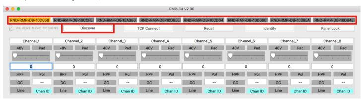
Once the desired RMP-D8 is selected, click the TCP CONNECT button. A successful connection is indicated by the device ID box color changing from orange to green as well as a "Connect Successful" message in the application dialog window.
