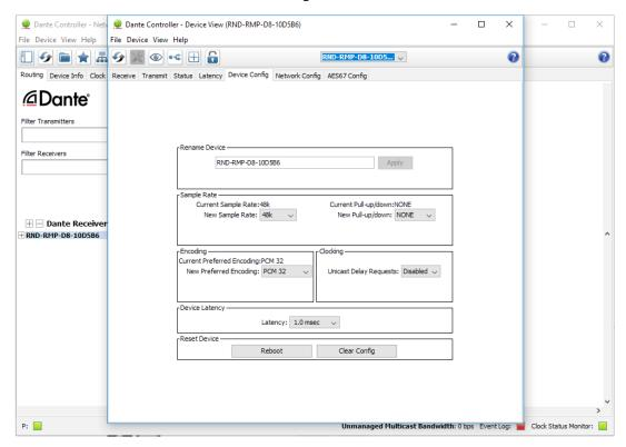
Within the Device Config Window, the user can adjust sample rate, bit depth, pull-up/pull-down and latency settings:
