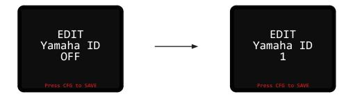
The RMP-D8 will then prompt the user to confirm the SAVE of the new Yamaha ID. Press the CONFIG button to save the Yamaha ID EDIT. The RMP-D8 will then show the new Yamaha ID prefix on the Dante ID menu screen. Press the CONFIG button once more to return to the main operational screen.
