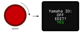
The RMP-D8 will then prompt the user to assign the Yamaha ID number. Rotate the ADJUST wheel to change the Yamaha ID number (in this example it was changed to ID 1). Press the CONFIG button to accept the Yamaha ID change.
