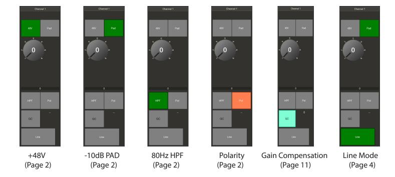
Note: When Line Mode is engaged in the application, the available Channel Gain range indicated is limited to +30dB, and PAD is automatically engaged.
