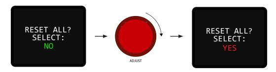
Rotate the ADJUST encoder wheel *one* detent clock-wise until the OLED screen prompts "YES." Press the RESET button again to accept the changes. The RMP-D8 will fully reset to its default state (all features disengaged and channel gain settings reset to 0dB).
