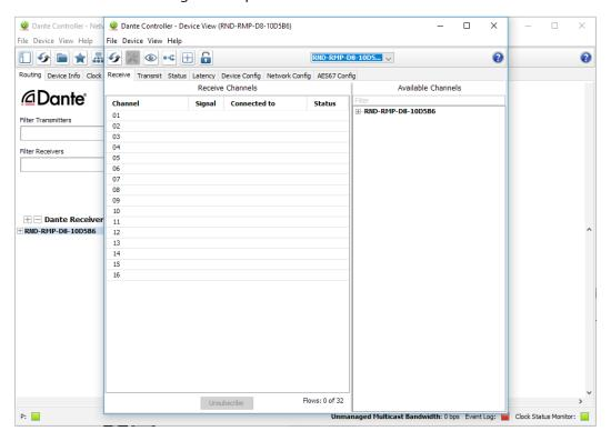
Within the Device View Window, click on the Device Config Tab:
