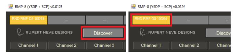
Once the desired RMP-D8 is selected, click the CONNECT button. A successful connection is indicated by the device ID box color changing from yellow to green as well as a "Connect Successful" message in the application dialog window in the lower left-hand corner.
