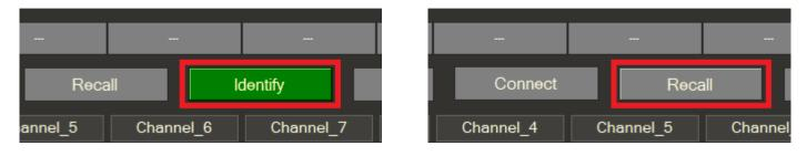
After verifying successful connection, the user should click on the RECALL button to recall the current status of all the features on the selected RMP-D8.
