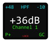
In addition to front panel status indication for a selected channel, the OLED display also shows configuration menus, which can be accessed by repeatedly pressing the CONFIG front panel button directly underneath the OLED display screen.
