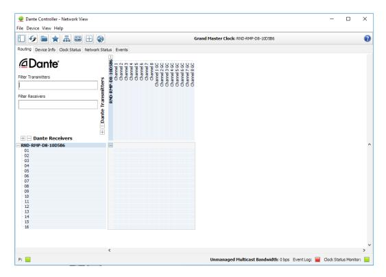
In order to change the RMP-D8 sample rate, bit depth, and pull-up/pull-down settings, double click on the RMP-D8 Device name in Dante Controller's routing tab to open the Dante Controller Device View Window.
